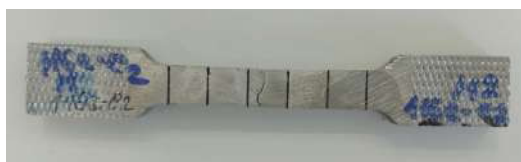
Fig. 3. Specimen after a static tensile test
