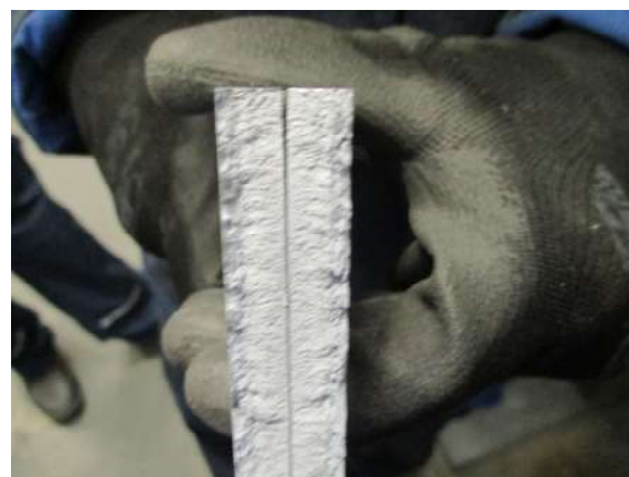
Fig. 6. Brittle fracture
