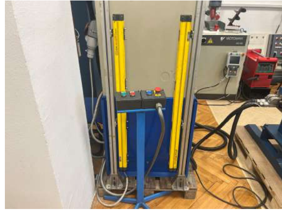
Fig. 12. External control and safety light curtain
