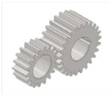
Fig. 5. Model of gears with 18 and 25 teeth
