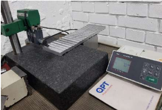
Fig. 3. Setup for surface roughness measurement
