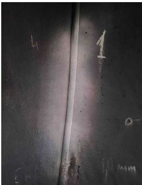
Fig.5. Liquid penetrate inspection performed on weld 1
