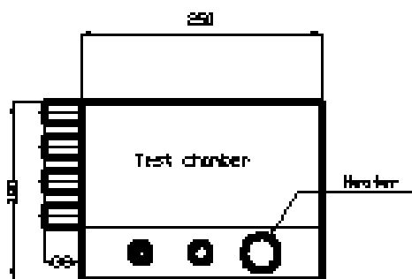
Fig. 1. Front side of the tank, with the heater position
