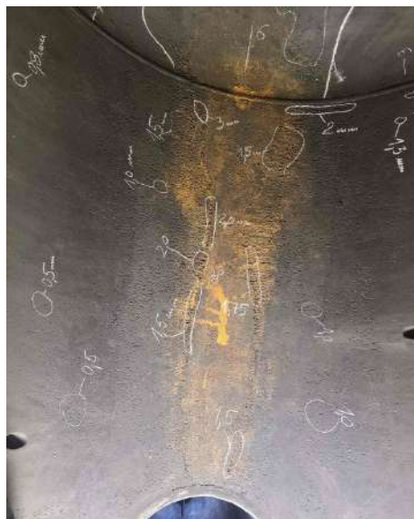
Fig.3. Pitting corrosion has been observed on the lower part of the shell (from 5 to 7 o'clock position) - majority of the pits are between 1.5 to 2.0 mm deep
