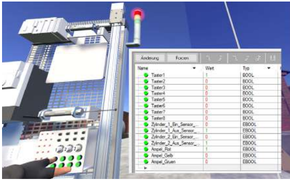
Fig. 6. Simulation of the activation of the first key in the VR world (left) and display of the state of variables in Unity Pro XL (right).
