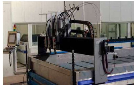
Fig. 2. Water jet cutting machine Water Jet NC 2525 D in SIJ ACRONI d.o.o.
