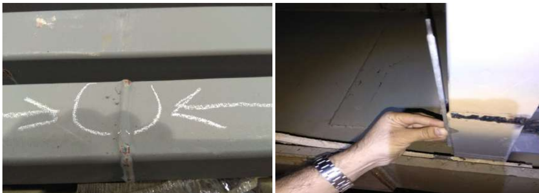
Fig. 4. Irregularity in the butt-welded joint (excess weld metal on the face of the weld)
