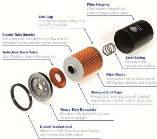
Fig. 1. General structure and main components of an engine oil filter [2]
