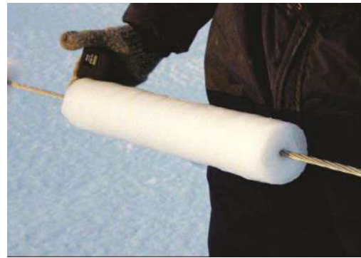
Fig. 4. Ice buildup on the rope [11]
