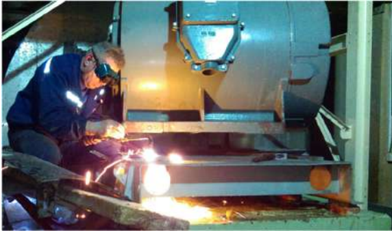
Fig. 6. Modification of the placement of the HV motor
