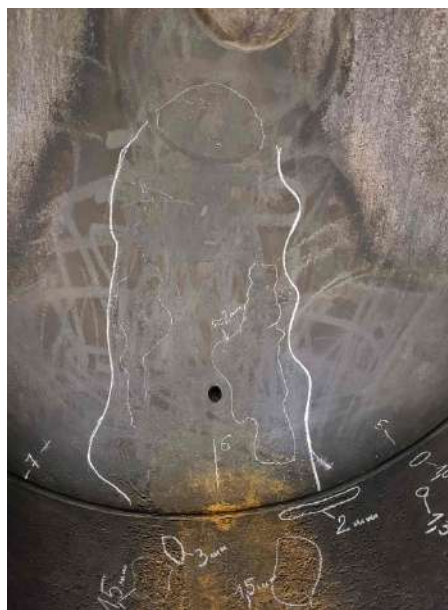
Fig. 4. Left head - close up view on the corroded surface (whole elliptical head has been scanned and minimum thickness was found to be 10.43 mm)
