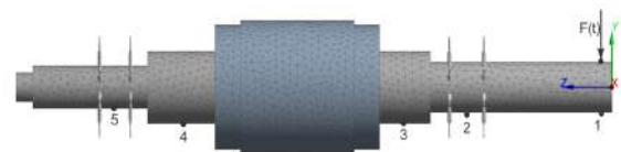
Fig. 2. Discretized model of shaft
