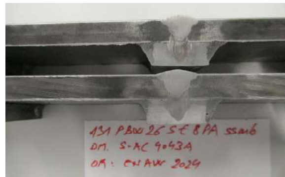
Fig. 2. Macrostructure of welded butt joint
