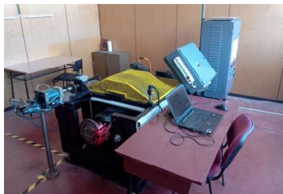
Fig. 2. Inertial brake dynamometer Brake Dyno 2020
