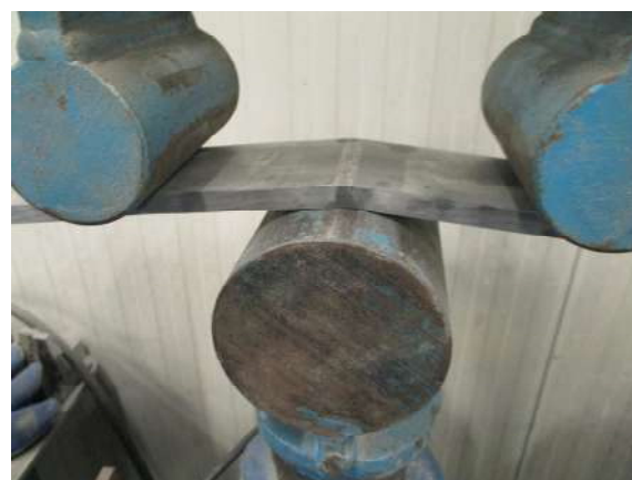
Fig. 5. Root bend test - moment of brittle cracking
