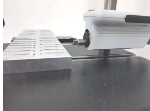
Fig. 6. Examination of roughness with the Mahr device
