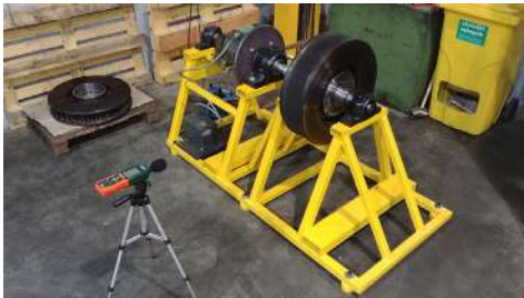
Fig. 6. Measurement of the air resistance of brake discs at rotation [63]
